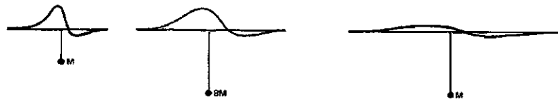
Figure 10.12 Depth/amplitude behavior of dipole anomalies (from [35]).
