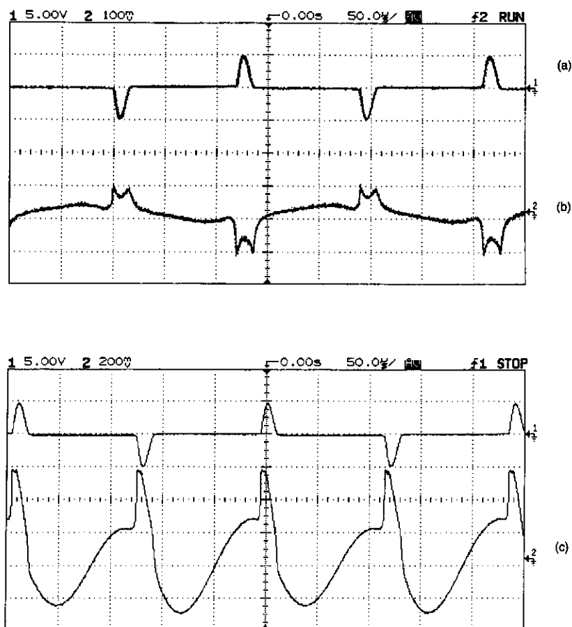
Figure 3.16 Waveforms in the tuned current-output fluxgate: (a) excitation current (0.5 A/div); (b) output current (20 \mu\text{A}/\text{div} ) for B_0 = 0 ; and (c) output current (40 \mu\text{A}/\text{div} ) for B_0 = 5 \mu\text{T} (from [93]).
